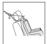
If the position you are using has an adjustable headrest or head restraint and you are using a dual tether, route the tether around the headrest or head restraint.
